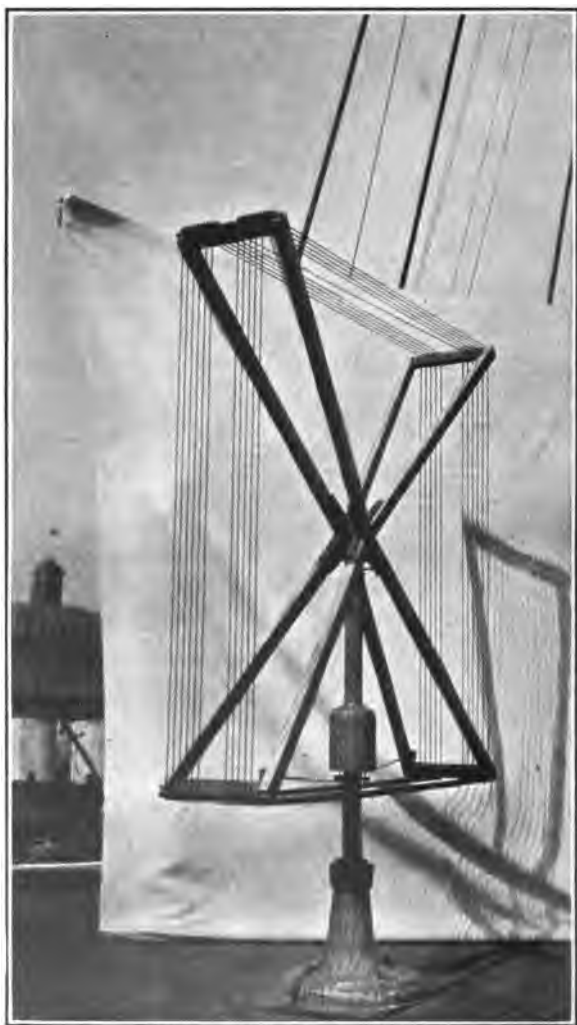
FIG. 179-E.—Bureau of Standards type of direction finder installed on lighthouse tender Tulip .
